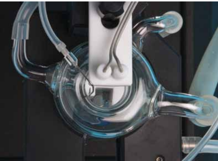
Tissue holders are designed for simple and accurate preparation mounting. As the tissue holder slides into the tissue bath, its size significantly lowers the volume of liquid in the tissue bath.
