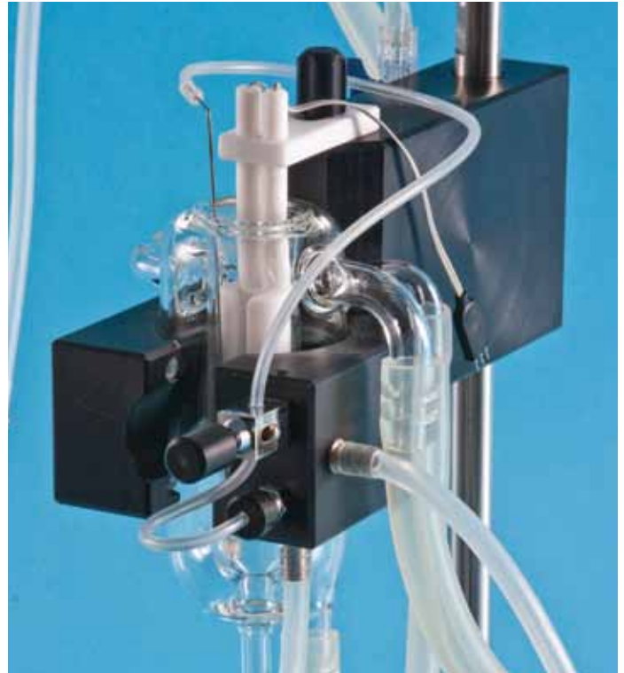
The mounting for each tissue bath provides solid support as well as ports for oxygenation control and fluid handling.
