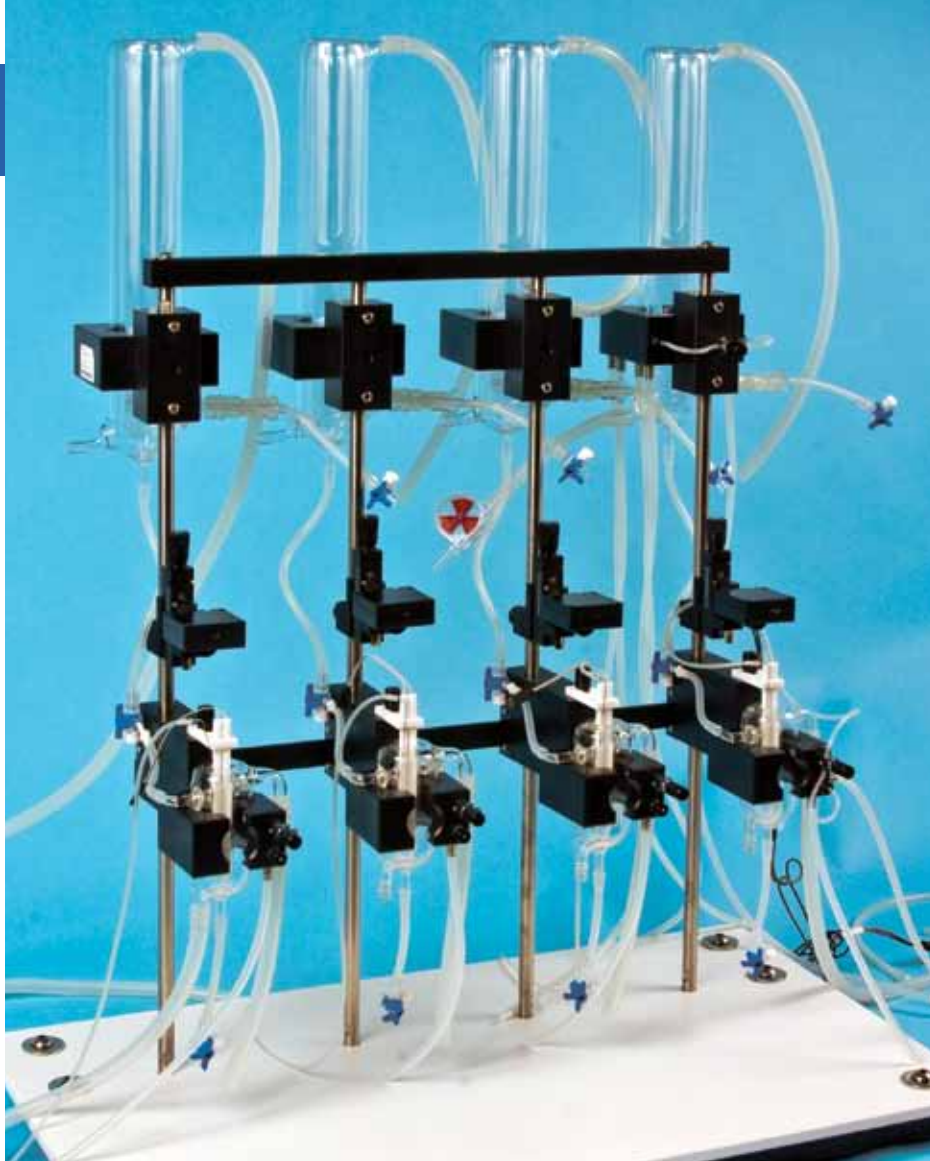
The SI-MB4 vertical tissue bath is shown with all four channels.
