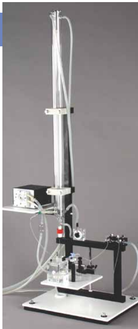
The Isolated Perfused Organ (IPO) system is designed as a perfusion system for isolated, small mammalian organs like the kidney, liver or mesenteric bed.
